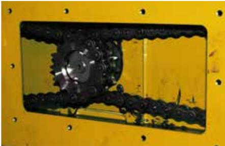
**EASY TRANSMISSION CHAIN TENSIONING**
